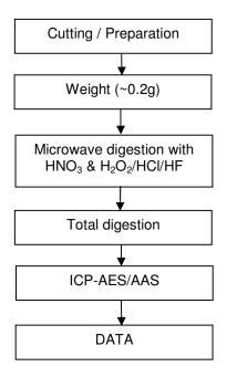
The samples were dissolved totally by pre-conditioning method according to above flow chart.
